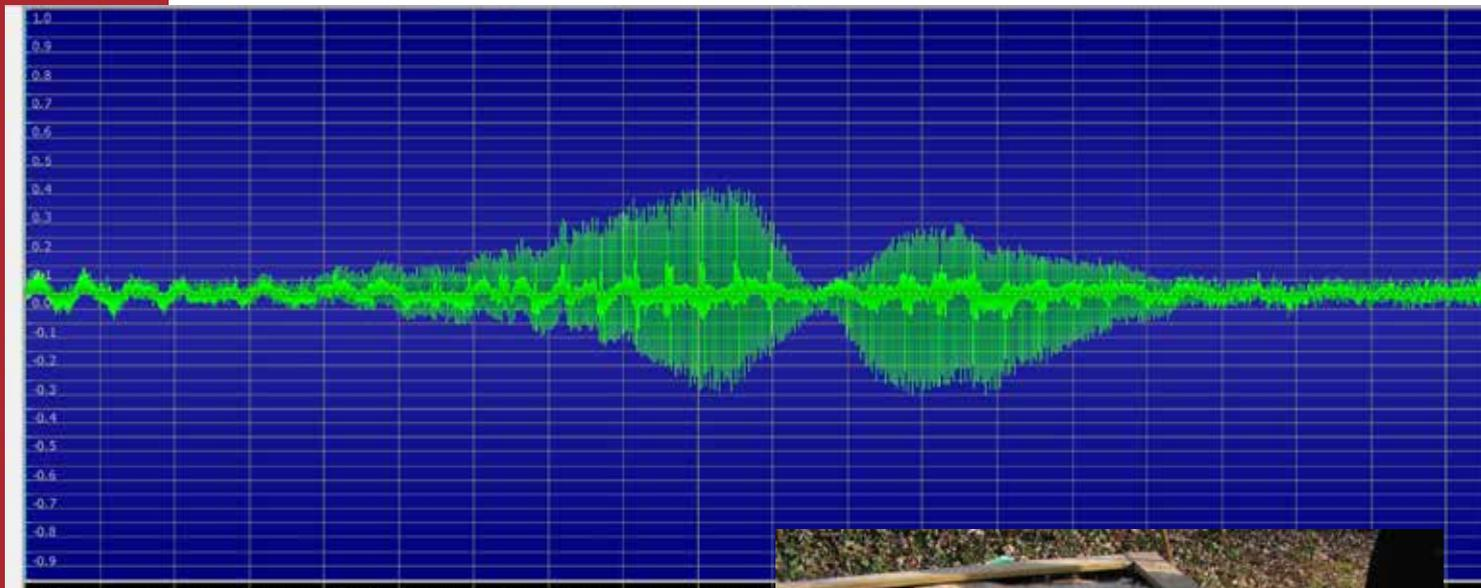
**Top:** In the landmine detector Marian developed, two microphones pick up sounds as the operator sweeps it across a minefield. A characteristic “swell-dip-swell” pattern indicates the presence of a mine.
